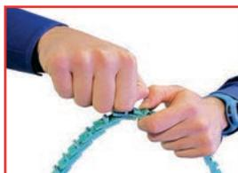
3. Put the belt with the tabs upwards and bend it as much as possible
