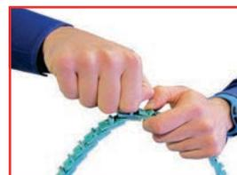
3. Ensure that tab will stay transversally to the belt's running direction; reverse the belt upside down to let it running on the tab side.
