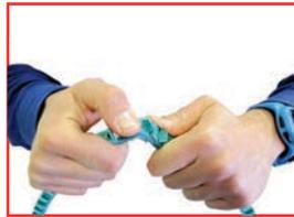
2. Flexing the belt as much as needed, twist and insert the second tab through the end link.
