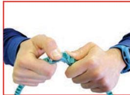
2. Twist one tab 90° to make it parallel to the belt; in this way you can pull the end of the link over the tab
